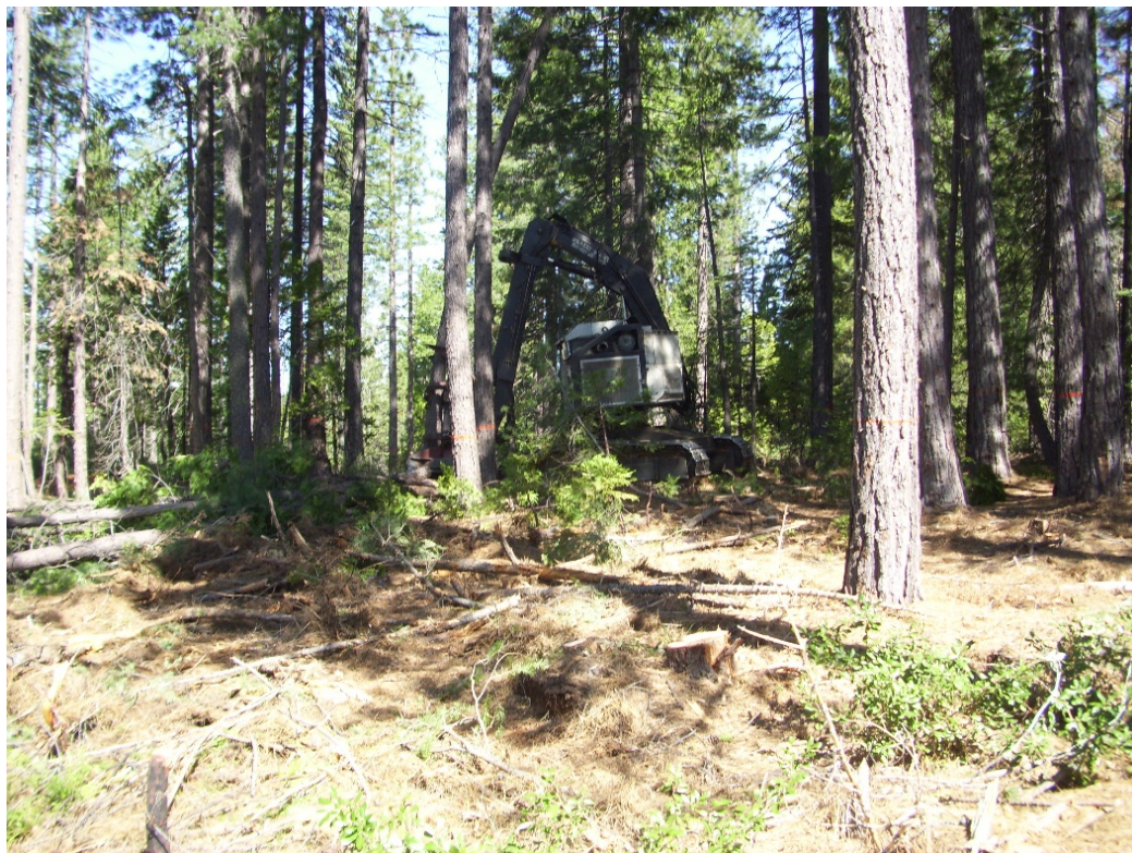
Figure F-1: feller-buncher operating in a biomass and sawtimber harvest unit.
