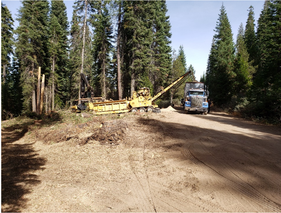
Figure F-2: example of an onsite chipping operation
